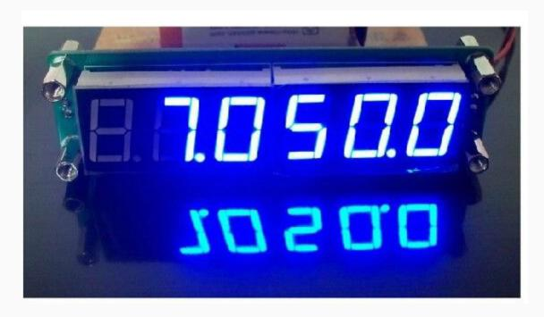
PLJ - 6 leds - A is designed for the HAM friends of cost-effective six LED display module, frequency is mainly used for transceiver equipment such as frequency values show, also can be used in the conventional frequency measurement.
