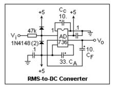
smooth the output. The values of the capacitors determine the averaging times and bandwidths, as is obvious. The values shown here are good for general service.  $C_A$  can range up to 150µF, and  $C_F$  up to 100µF, if desired. The **AD736** will handle crest factors up to 5.
